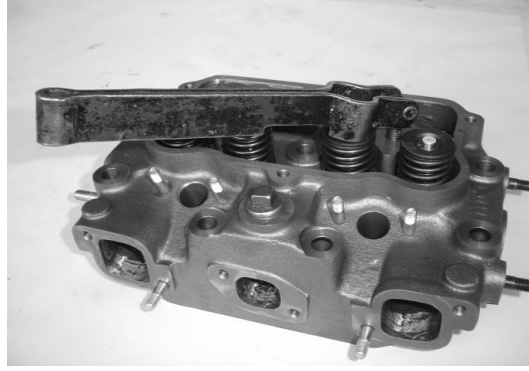
Valve Spring disassembly with tool
